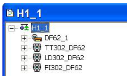
Figure 19. 17 – Devices added into the Fieldbus channel
